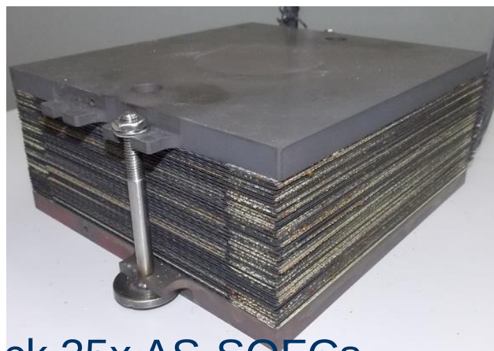
Modular stack 35x AS-SOFCs
